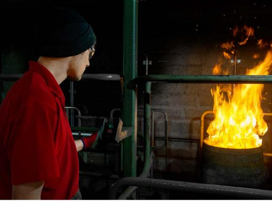
whisky? After coopers have selected the staves and assembled a cask, they will toast and/or char it to the desired level to obtain different balances of certain flavour compounds for the spirit to extract. Wood is mostly composed of lignin, which once exposed to heat degrades into a large variety of flavour-active molecules. We know this is the process by which vanillin and its dreamy sweetness is created.
